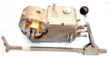
We supply new selector rods with the gear box because the original gear-lever can be badly worn and, with the accurate gear changes required, the selector rods have been designed to reduce twist and provide minimum clearances. The selector rods and gear-lever are made from stainless steel. The gearboxes are now completed. We also produce our own modified cross-shaft. These have now been completed and tested. The gearboxes can be supplied with the modified cross-shaft.
