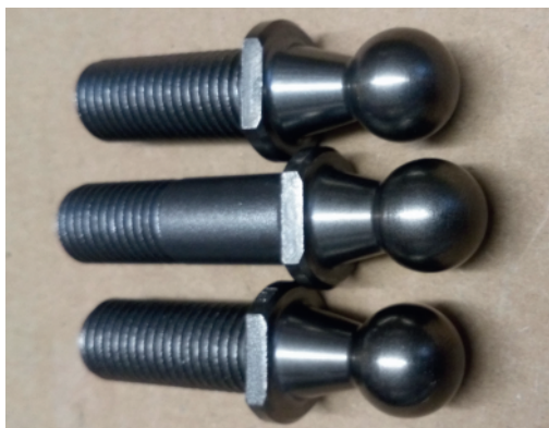
Above: Early F type track rod end Left: Twin and F type (longer shank) ball pillars
