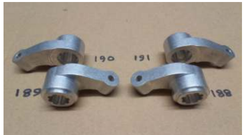
New rocker arms, machined from billet
