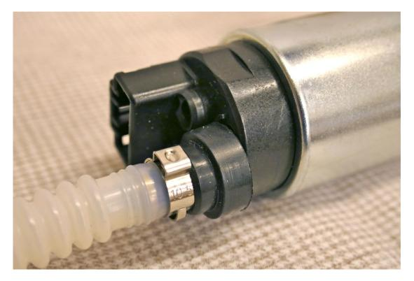
On the other end of the pump module, fit the pre-prepared rubber foot, white plastic stand off and inlet filter in the orientation shown.
