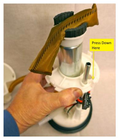
Reassemble the pump and collector pot.
