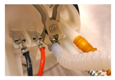
• Fit the wiring loom to the pump, twist the new loom around the module 'leg' like the original and connect the spade connectors.
