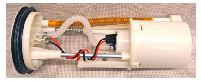
The pump assembly is now complete and it can be refitted into the tank.
