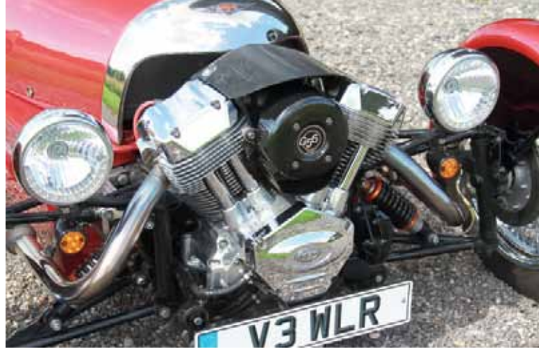
The S&S is a thumping brute of an engine, two air-cooled cylinders producing 82bhp at 5250rpm and 103lb.ft at 3250rpm in Euro 3 trim.
