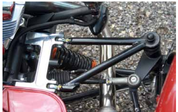
The aluminium bracket at the inboard end of the upper wishbone corrects the steering geometry and drastically reduces bump steer.
