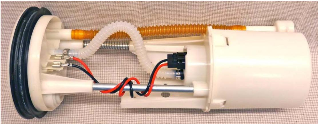
The pump assembly is now complete and it can be refitted into the tank.
