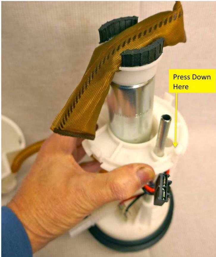
Reassemble the pump and collector pot.
