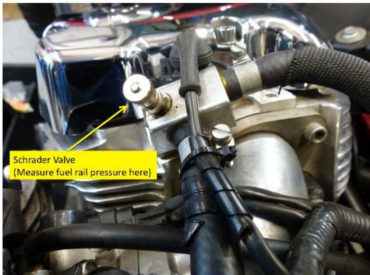
There is a fuel rail pressure test point on the RH fuel injection nozzle, a Schrader type connector. If you have the Urban Cooling Kit you will need to lift it for access. With the pump running, the pressure should be 58 psi.
