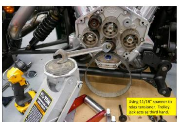
Now hang the belt over the new pulley with the writing on the belt the 'right way round', i.e. so that you can read the printing.
