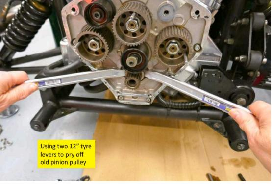
With the old pulley removed, it's time for a good clean up of the chamber. Check the tensioner & idler pulleys for 'pick-up' and clean if necessary.
