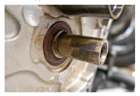
Do a trial fit of the new pulley onto the shaft to make sure that you've cleaned up the shaft sufficiently. It should be a reasonably snug fit but not too tight.
