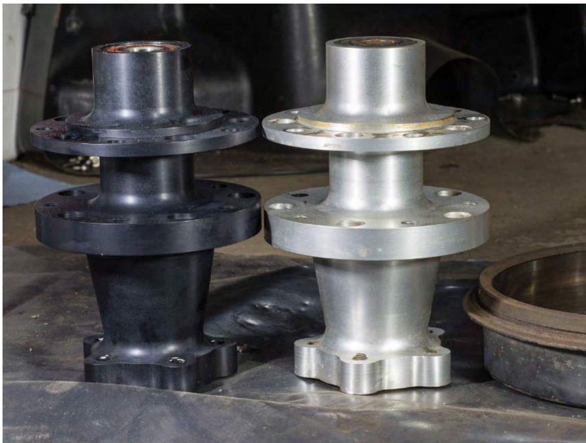
Later style hub on left – anodised black – showing the change in wheel mounting flange position when compared to the old style silver hub.
