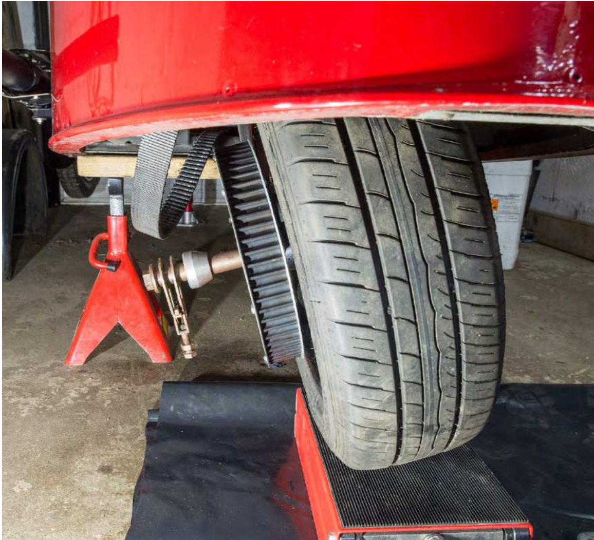
Spindle inserted through hub.
