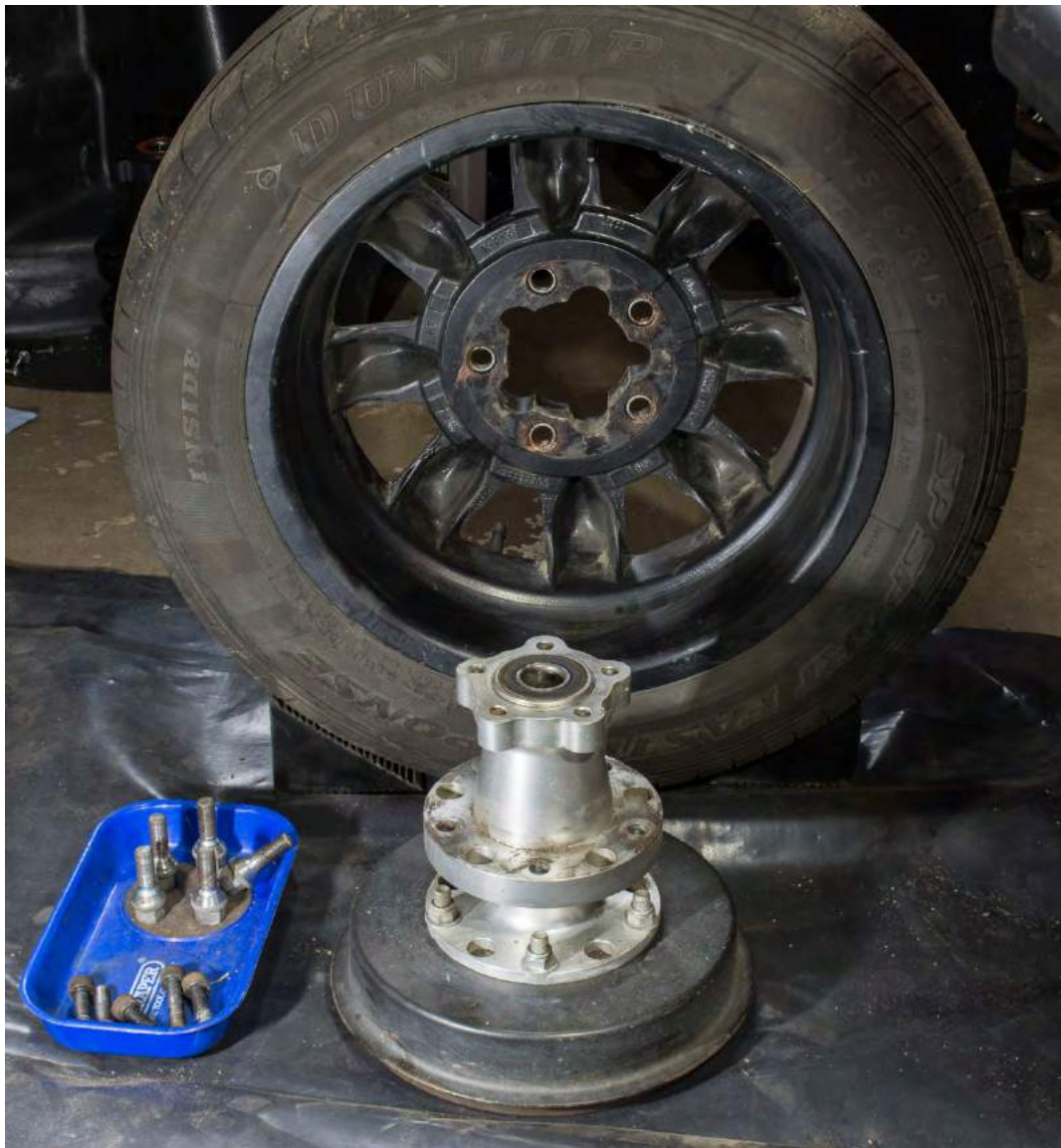
Hub still with brake drum attached and the side of the wheel it attaches on to.
