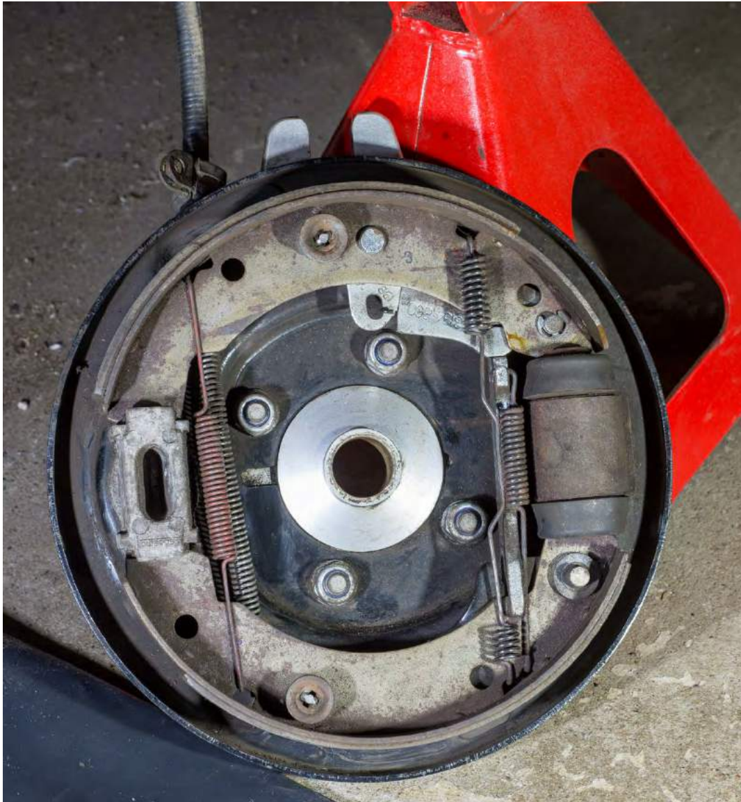
Inside of the drum brake mechanism. On this occasion I just dusted it out and gave it a wipe with brake cleaner, maybe next time I'll take it apart and grease the pivot points.
