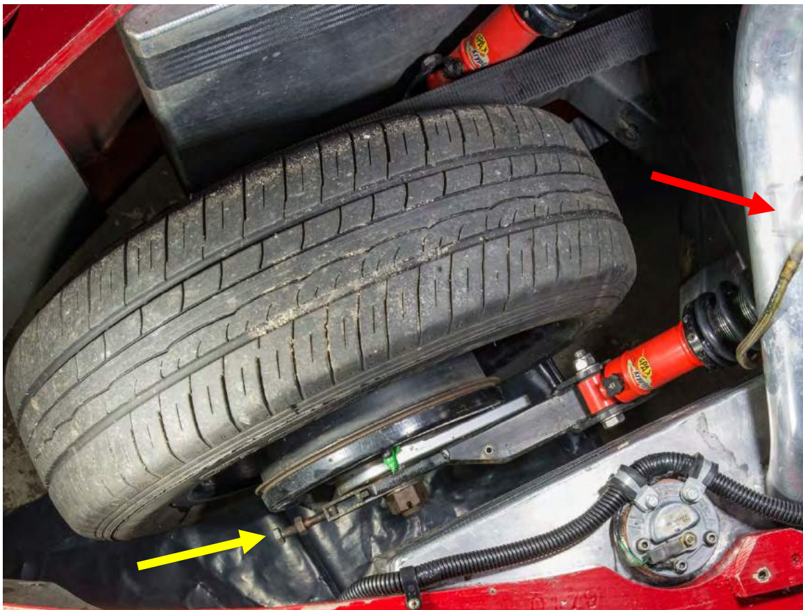
Brake hose P-Clip on swingarm removed and disconnected from drum, the end bagged and taped and secured up out of the way to the fuel filler pipe (arrowed in red). Green tape protecting the brake hose fitting on the drum backing plate. Belt tension adjusters backed right off (both sides) (arrowed in yellow). Split pin removed from spindle. Not visible; P-Clip also removed from hand brake cable on underside of swingarm and two tie-wraps cut.
