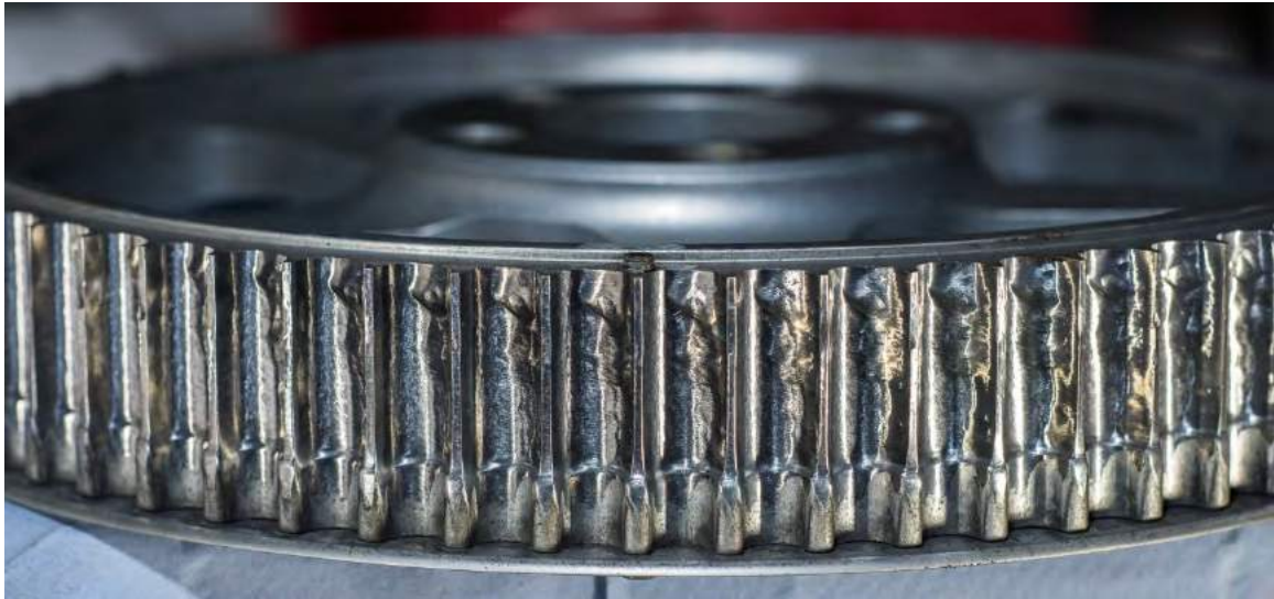
The aluminium sprocket after about 17000 miles.
