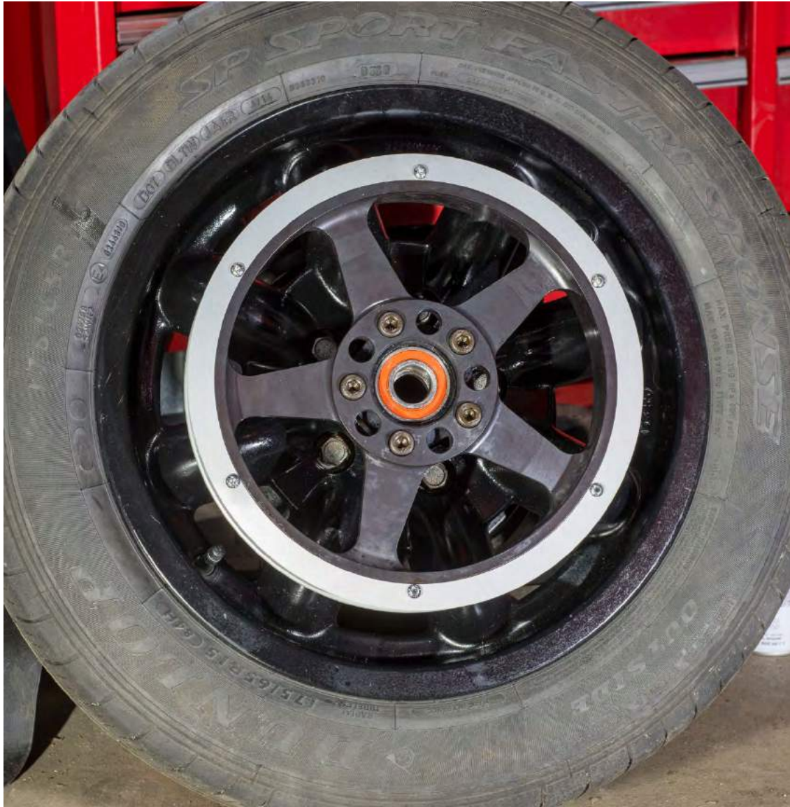
New steel sprocket mounted on the wheel assembly.
