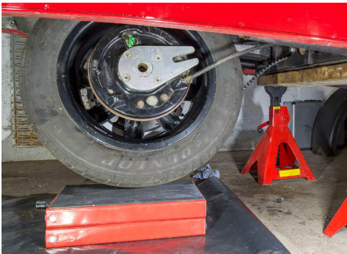
Brake mechanism placed back into the drum with the reaction fork pointing forward ready to engage with its boss on the swing arm.
