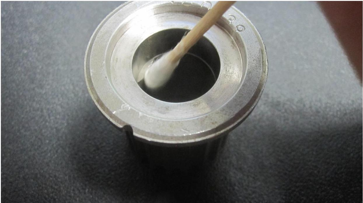
It is important to apply the loctite in this manner so it smears across the crankshaft surface when installed.
