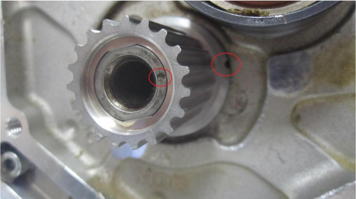
Remove all timing dowel pins from the camshafts pulleys, using the spanner wrench or 3/4" socket to relieve force if the pulley is under load.
