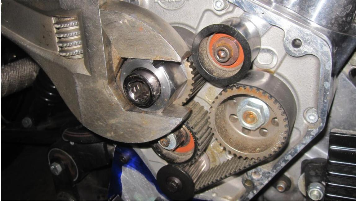
Remove pulleys if possible. Do not use tools, if the pulleys are tight, skip to the next step.
